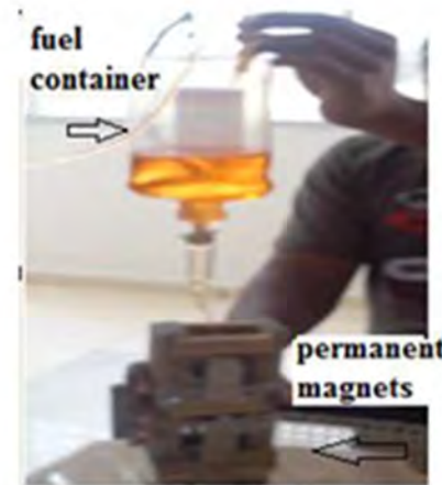
Fig. 9. (a) De-clustering of hydrocarbon molecules, (b) Experimental setup for analysis of the effect of magnetic field on the viscosity of petrol [70].
